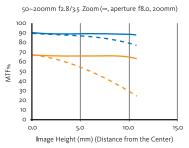
Innovative design, the finest materials and cutting-edge manufacturing techniques result in measurably superior image quality. In these MTF charts, the blue lines measure contrast while the yellow lines track resolution, measured from the center of the image to the corner (left to right on chart). When compared to lenses with similar apertures and comparable focal lengths, these higher curves indicate superior lens performance.
