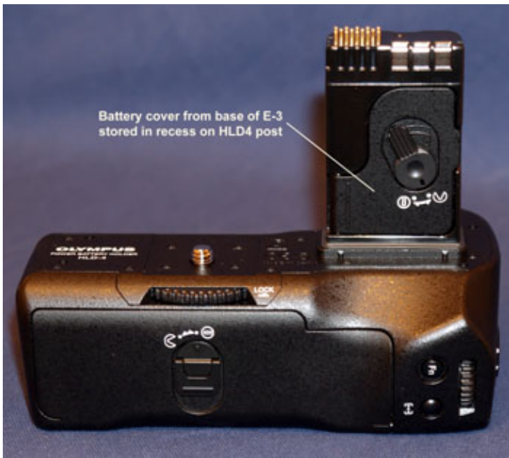
HLD4 rear elevation - here is battery door to access space for 2 x BLM1's. Also notice the extra Fn button and AF control.
